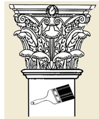
Fig. C – Apply a high quality primer before painting.
